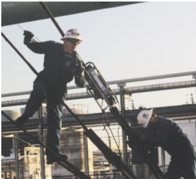
Electromagnetic instrumentation installed on a guy for inspection
